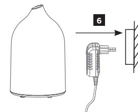
**6** Plug the adapter into a power outlet.
