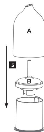
**5** Replace the inner cover (B) as well as the ceramic cover (A).
