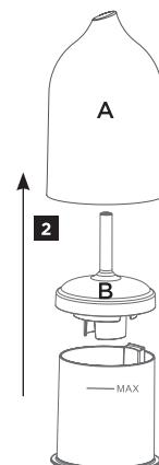
**2** Gently remove the ceramic outer cover (A) and the inner cover (B).
