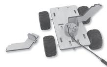
04 - Install the wooden pieces together as shown in the figure. The installation methods of left and right sides are the same.
