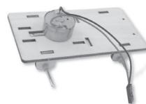
02 - Install the motor to the position shown in the figure with a short screw.
