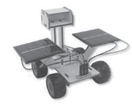
08 - Insert the wires of motor and two solar panels into the pin headers. The red lines are inserted into one side, and the black lines are inserted into the other side (The motor wires can be inserted freely, as it only affects the car move forward and backward.).
