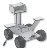
07 - Put double-sided tapes on both sides of the two small wooden pieces as shown. Then install the pin headers to the position shown in the figure with long screws.
